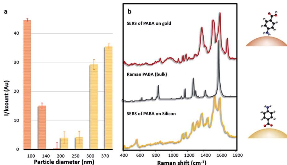
Fig. 4 (a) Intensities and (b) SERS spectra of PABA excited at 785 nm on colloidal dispersions of gold (100–400 nm) and silicon (200–370 nm) particles. Gold (red) and silicon (yellow).
