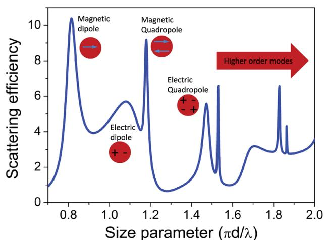
Fig. 1 Scattering efficiency of a single silicon spherical nanocavity as a function of the size parameter. We have assumed a constant value for the refractive index of silicon ( $n = 3.7$ ).
