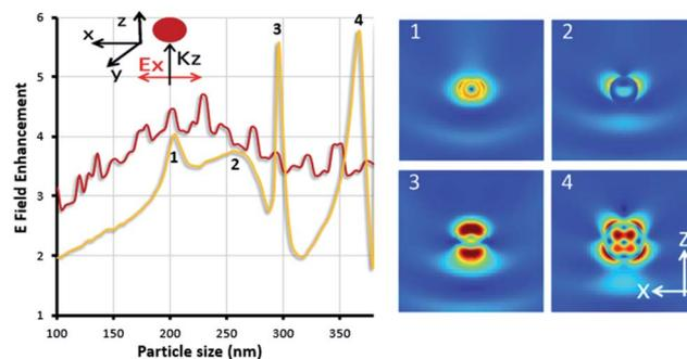
Fig. 2 Field enhancement around spherical particles of both silicon (yellow line) and gold (red line) as a function of the particle size when they are shined with a laser with a wavelength value of 785 nm, for particles embedded in air and the field distributions of the numbered peaks in the graph: (1) magnetic dipole, (2) electric dipole, (3) magnetic quadrupole, and (4) electric quadrupole modes.
