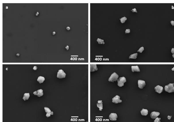
Fig. 3 SEM image of SiNPs obtained through mechanical milling of silicon powder together with further particle separation through a colloidal sedimentation process: (a) 200, (b) 260, (c) 300 and (d) 370 nm.
